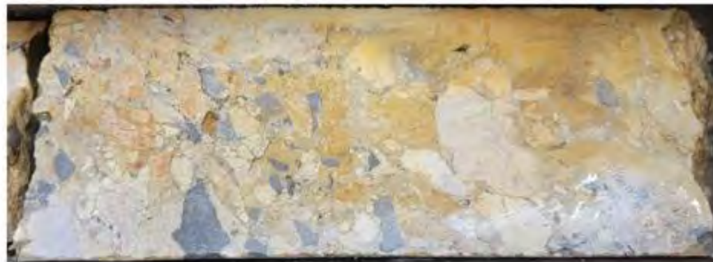
Underlying breccias are cherty and clast-supported and grade downward into crackle breccia and eventually into unfractured limestone
